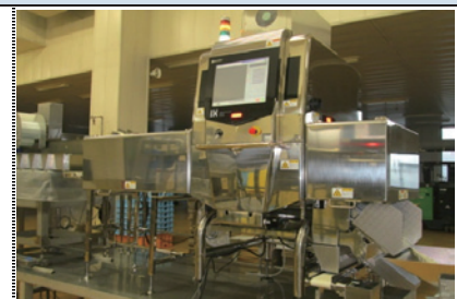
X-ray foreign matter detector: Prevents contamination and removes foreign matters
